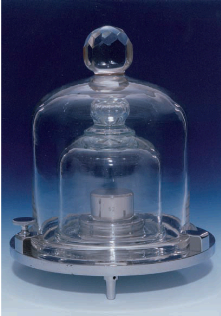
The national prototype of the kilogram of Germany - No. 52 -
