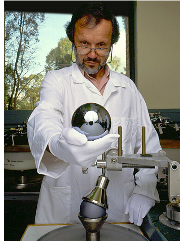
1 Kg single-crystal silicon sphere the roundest man-made object in the world
