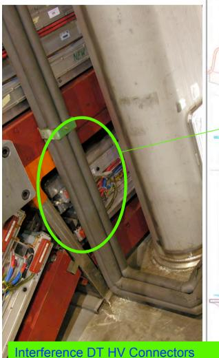
with piping on Sec. 3. Drawings updated. Modification foreseen before Magnet Test.
