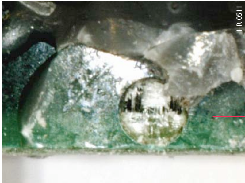
Fig. 4: Same rear face of the HVC, viewing orthogonally to the PCB. It evidences that the HV pad of ~1.3 mm diameter is located dangerously near the PCB border. The red line shows here where the GND starts in the inner layers of the PCB (darker area).
