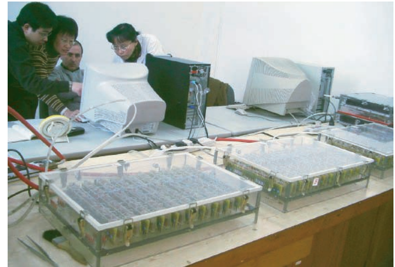
HV test; at front the 3 test jigs loaded with HVBs.
