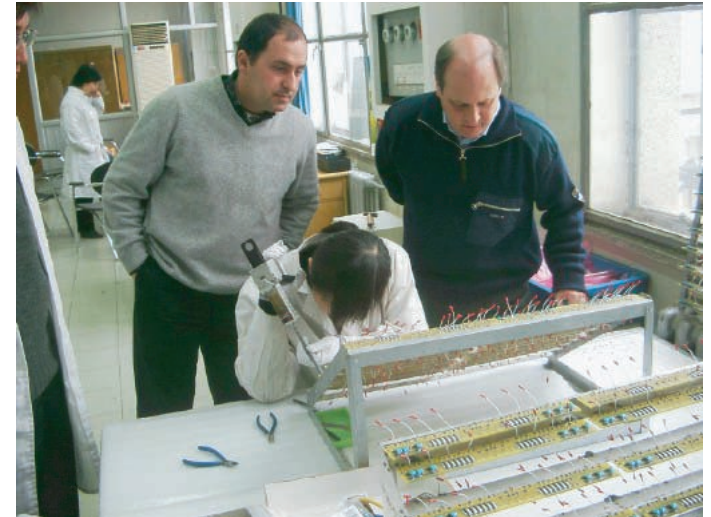
After soldering components, deposit glue
