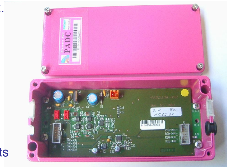
A PADC board in its housing box, ready for installation.
