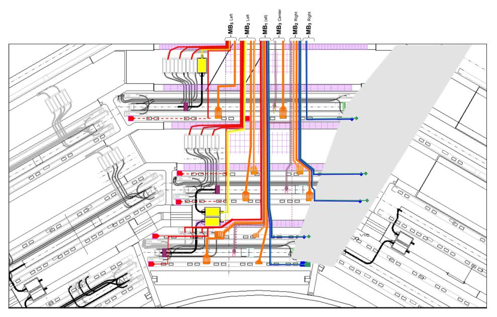
MB<sub>123</sub> and RB<sub>123</sub> ZpL's Radial Cabling by channels (*First proposal* to be used in Wheel +2 Sector 4/10)
