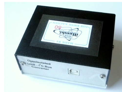
Interface USB-I2C, as made at Debrecen
