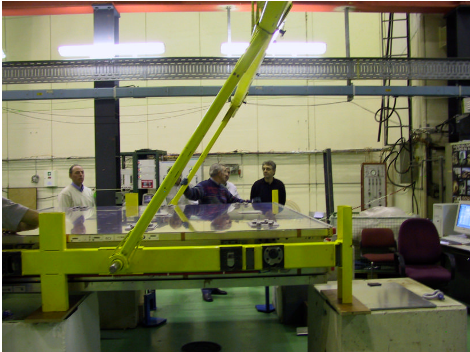
MB2 with one RPC already installed
