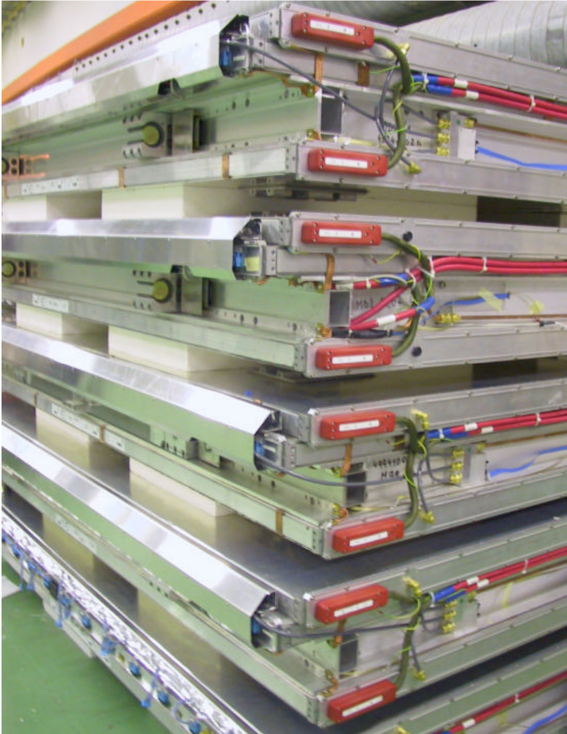
MB2 with Theta cabling, cooling and carters
