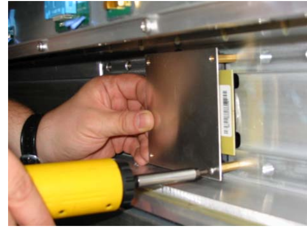
Installation on the chamber: fork, cabling, cover
