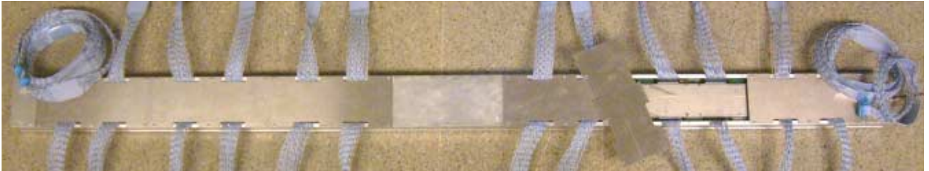
MB2 minirate prototype with readout electronics under test in CIEMAT
