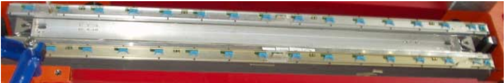
MB2 minirate prototype with readout electronics under test in CIEMAT
