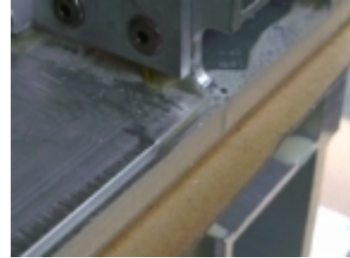
Glue rests in groove are visible; also dirt in profiles (mainly glue rests, from grinding).
