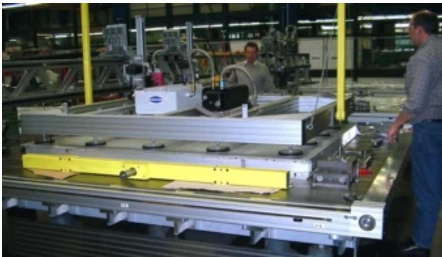
Placing a panel on the flat table for measurement.
