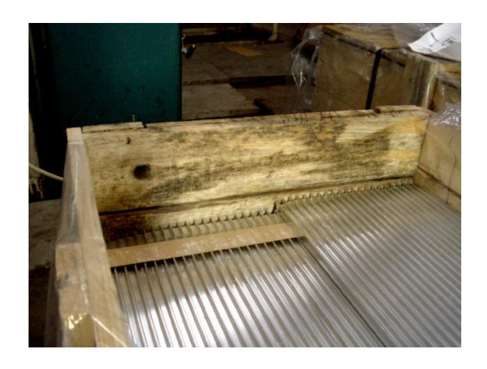
Box with bad plastic lining. Aluminum oxide visible on cardboard spacer.
