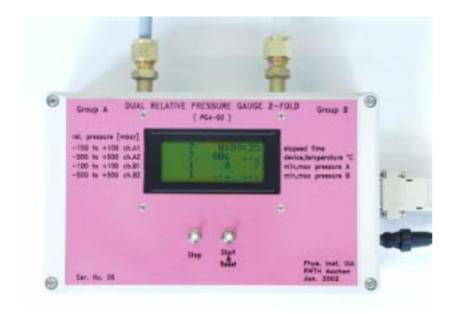
View (left) of the measuring device with two channels, each with a 100 and a 500 mbar (+ and -) range differential pressure transducer. 8-bit ADC inside. Readings either from the display or via computer (bottom, software by M. Sowa).
