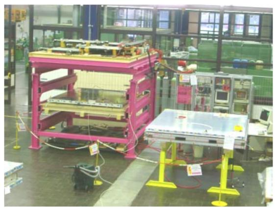
Bench for tests with cosmics (pink); can house 3 DTs or up to 9 SLs. HV supply, patch panel, TDCs, DAQ in racks. SLs undergoing HV test in gas are on external (yellow) support.
