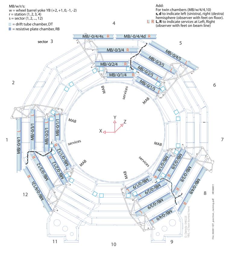
Naming of CMS DT chamber position: The convention is to look at the FrontEnd side of the chambers, having the feet on the beam axis and to name the chamber POSITION in the form MB/wheel/station/sector.
