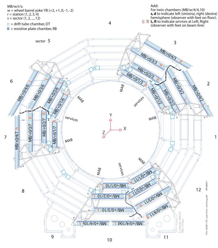
Naming of CMS DT chamber position: The convention is to look at the FrontEnd side of the chambers, having the feet on the beam axis and to name the chamber POSITION in the form MB/wheel/station/sector.
