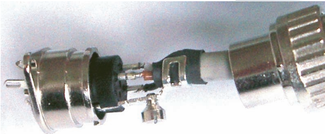
Fig.7: Cable for +6 V supply to PADC, far end. This connector is plugged at the LV patch panel located on the front face of the magnet yoke iron "wheel", close to the front-end of the chambers. On the two photos the connector on the cable is open and is plugged into his matching patch panel connector, to show the details of the assembly. The LV cable for the minicrate is connected to the same patch panel. At this end of the PADC_LV cable the shield remains dc-floating; inside the patch panel it is connected capacitively to the shield of the cable from the supply.
