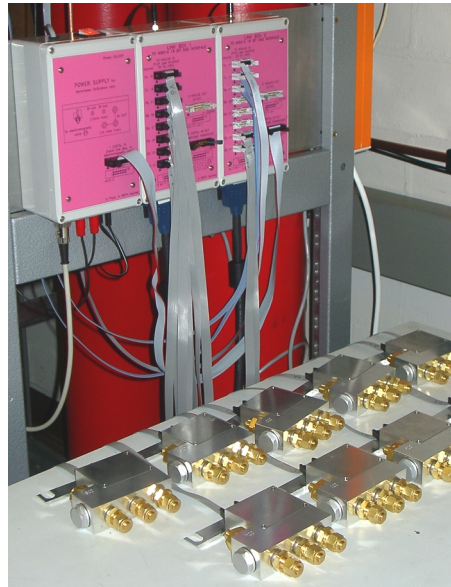
Fig. 2: Side of the calibration rack, with 10 manifold units with integrated pressure sensors to be calibrated. Each unit is connected via one flexible tube and one flat cable.
