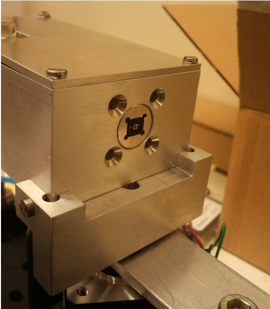
Figure 4.4: Picture of the SiPM mounted on top of the rotating axis of the aluminium box. Later, the aluminium box have been painted with a matt, black varnish.
