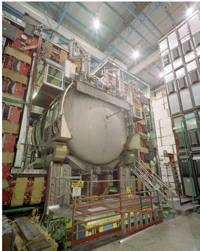
Figure 2.6: A Photo of one of the DØ End cap Calorimeters, in the middle one can see the beam pipe[9].
