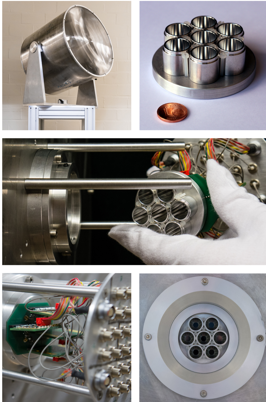
Figure 5.12: Photos of FAMOUS (preliminary design with a seven pixel camera). Top left: Telescope on an altitude-azimuth mount. View on the aperture with the Fresnel lens. Top right: Small focal plane array with seven Winston cones. Middle: Mounting of the seven pixel camera. The SiPMs (not visible) are soldered onto the green printed circuit board (PCB). Bottom left: Camera compartment with detached cylindrical housing. The vertically orientated PCB carries the SiPMs and the temperature sensors. The piggyback connected PCBs hold the amplifiers (up to eight channels per PCB). Each SiPM has its own output channel (7x4 channels, gray cables and small connectors, signals of one camera pixel are not summed up at the focal plane electronics). Communication and bias voltages are provided via the big connectors and the colored cables. Bottom right: View onto the seven pixel camera. At the exit apertures of the Winston cones the UV band-pass filters are mounted in front of the SiPMs (not visible).
