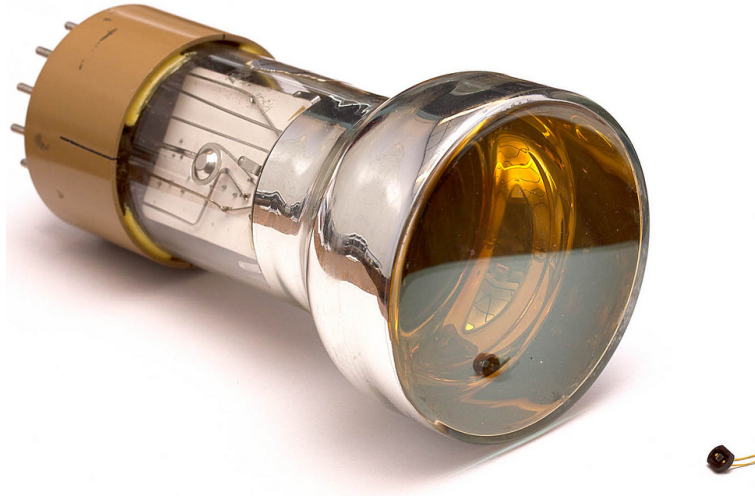
Figure 5.1: Photo of a 3 inch photomultiplier tube (left) and a silicon photomultiplier (right). The active area of the silicon photomultiplier is 1 \text{ mm}^2 . Taken from reference [125].
