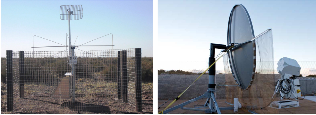
Figure 3.11: Left: Photo of a radio detector station of AERA. Visible in the center of the picture are two active bowtie antennas perpendicular to each other. An antenna for communication is mounted on top. The box at the bottom is covered with solar panels and houses the electronics and batteries. Taken from reference [84]. Right: Photo of AMBER, one of the microwave detector prototypes of the Pierre Auger Observatory. In the focus of a 2.4 m off-axis parabolic dish a camera with 16 pixels is located. The pixels are commercial C-band and Ku-band microwave receivers. Taken from reference [87].
