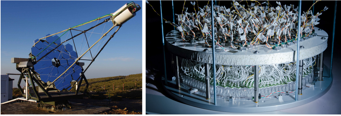
Figure 5.13: Left: Photo of the FACT telescope at the Observatorio del Roque de los Muchachos on La Palma, Canary Islands, Spain. Right: Photo of the assembled sensor compartment of FACT. From bottom to top: the front flange with the entrance window, the Winston cones, the SiPMs (white packaging), the printed circuit boards (green) for the co-axial cables (white), and the insulation plate. The black connectors on top are for the signals of the SiPMs, the three-pole cables (white-black-orange) for the bias supply. Other colored cables (yellow-purple and red-green-white) connect the temperature and humidity sensors. Both photos taken from reference [149].
