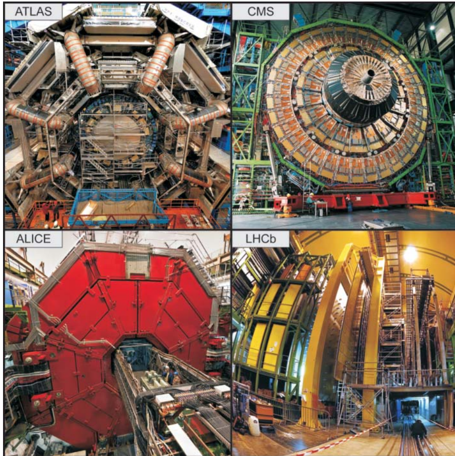
Figure 3.4.: The four main LHC detectors. The aim of the two largest experiments ATLAS and CMS is primarily the search for the Higgs boson, ALICE is particularly designed for the study of heavy ion collisions and LHCb investigates the B-physics (Photographs from [21]).
