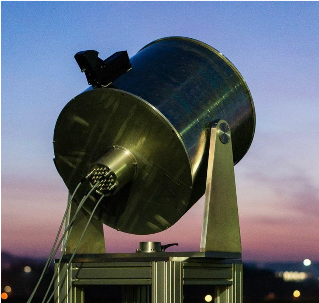
Figure 1.6: This photo (taken early in 2013) shows the FAMOUS 7 fluorescence detector prototype from behind. Four cables are attached to the front-end electronics of FAMOUS 7 . The Fresnel lens cannot be seen on this photo. The photo has been taken by Tim Niggemann.
