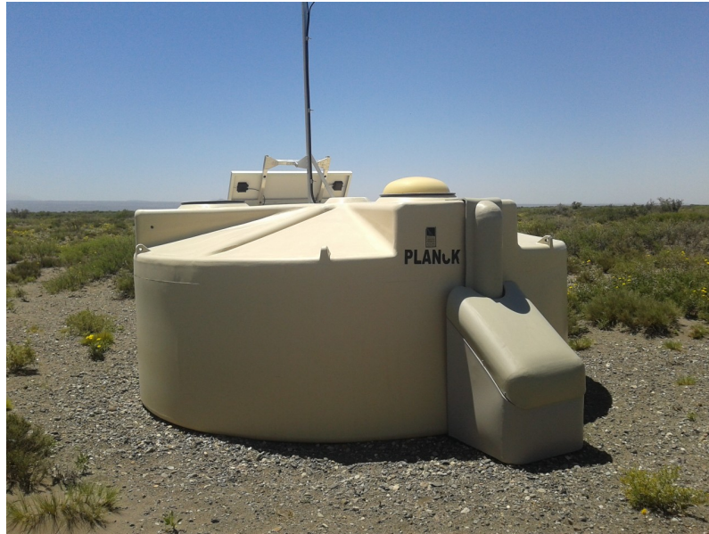
Figure 1.3: A photograph of a typical surface detector (SD) station taken by the author. This detector type is based on the water Cherenkov principle. Particles passing the tank faster than the speed of light in water will generate Cherenkov light cones. This is measured by 3 photomultiplier tubes.
