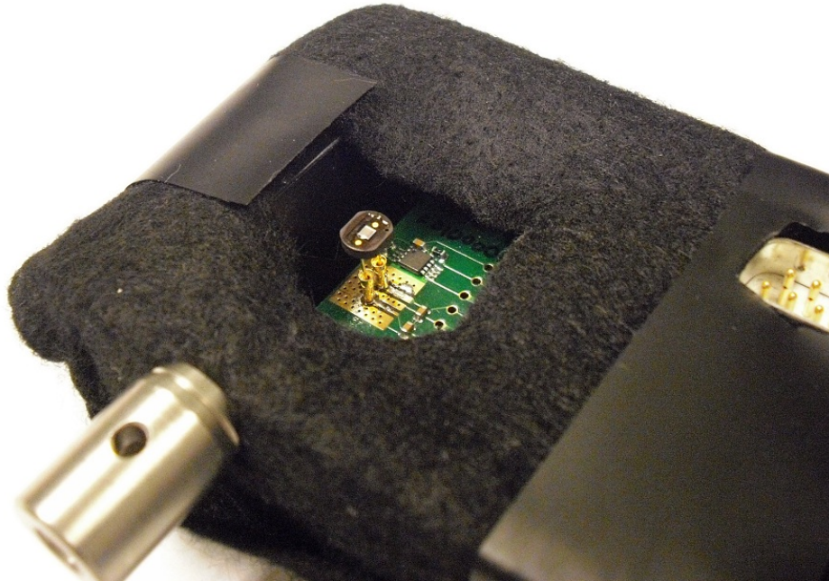
Figure 3.8: Frontend electronics designed by F. Beißel (III. Phys. Inst. B, RWTH Aachen University) and silicon photomultiplier manufactured by Hamamatsu (HAMAMATSU S103612-11-100C) conditioned for the relative PDE measurement.
