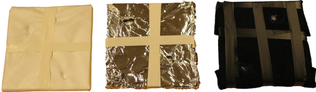
Figure 4.5: (10 \times 10 \times 0.8) \text{ cm}^3 scintillators wrapped in Tyvek, Aluminium foil/dull side, Black felt (from left to right)
