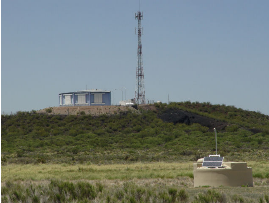
Figure 4.1: This picture shows one of 1600 Surface Detector stations in the front and one of four standard Fluorescence Detector buildings with its communications radio tower in the back.
