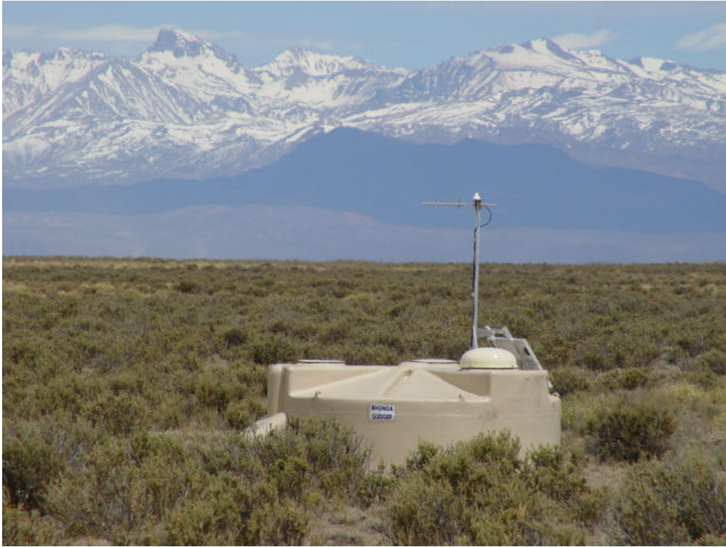
Figure 4.4: This picture shows one of 1600 Surface Detector stations deployed in the pampa.
