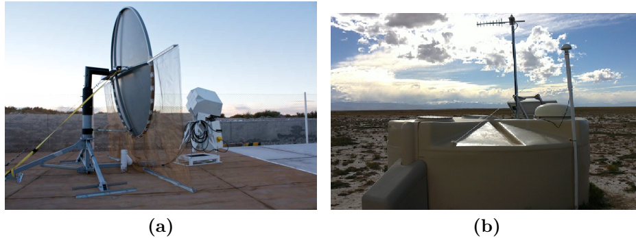
Figure 4.23: Prototype experiments for microwave detection of air showers. 4.23(a) shows the antenna dish of AMBER installed close to the HEAT telescopes as an example for several experiments. 4.23(b) shows a SD station with an installed EASIER antenna (right mast, c.f. figure 4.3 and 4.4). Pictures from [123].
