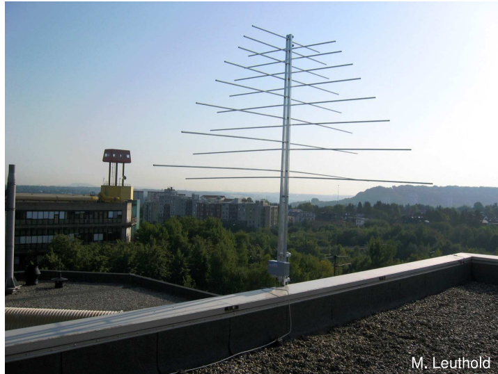
Figure 15: Picture of the LPDA mounted on top of the Physikzentrum in Aachen.
