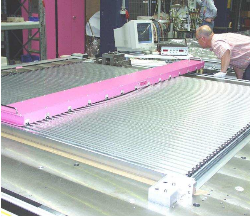
Figure 3.7.: One of the tests that is done for every layer of wires is a measurement of their mechanical tension. Via a contactless measurement of the resonance frequency, the mechanical tension of every wire is determined.
