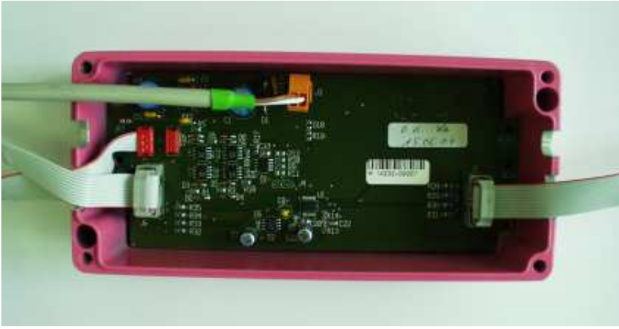
Figure 5.4.: The PADC board in its pink housing. The lid, carrying a label with information on the board, is not shown here.
