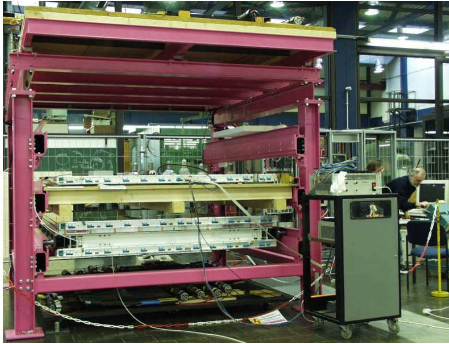
Figure 3.8.: The test stand in Aachen. Muon chambers and single Super Layers are tested with muons from cosmic rays.
