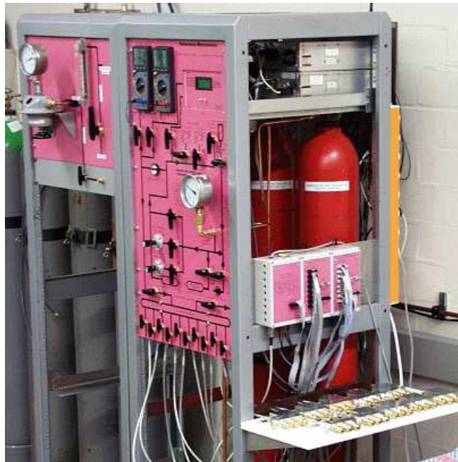
Figure 4.3.: The gas teststand, used for the calibration of the pressure sensors. The manifolds, up to 10 per cycle, are placed on the white plateau in the lower right corner.
