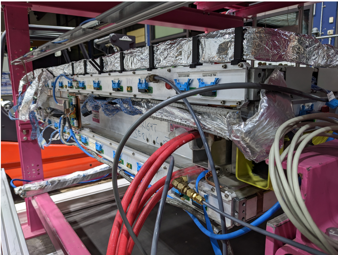
Figure 2.5: A picture of an MB1 chamber in the III. Physics Institute A at RWTH Aachen University. The vertical gap between the blue connectors serves as a storage for the Minicrate.
