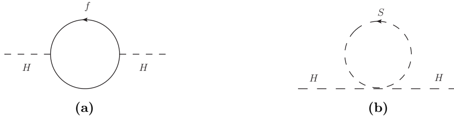
Figure 1.6.: Higgs boson with loop quantum corrections from a fermion 1.6a and a scalar 1.6b
