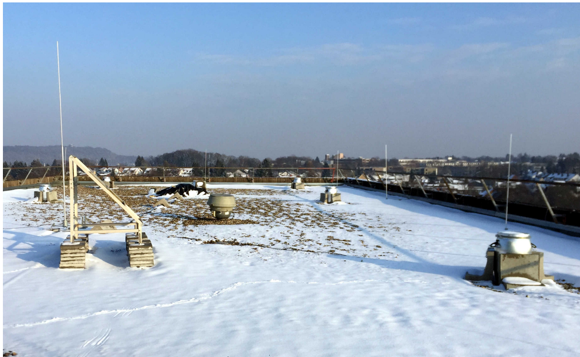
Figure 9.12.: Photo of the air shower array located on the roof of the physics department in Aachen. It consists of six stations. Each station consists of a barrel protected against light leakage with a layer of adhesive aluminum tape at its outside. The MiniAMD detector is located under a black pond liner in the middle of the array.
