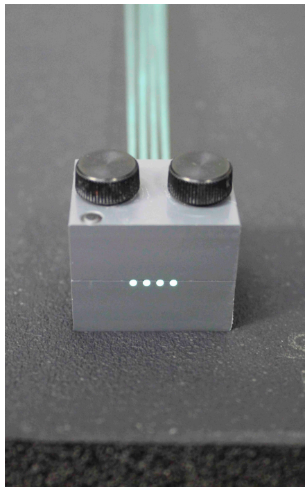
(d) The acrylic block contains four polished WLS fibres. A homogenous surface has been achieved. However, the outer cladding may be still damaged after polishing.
