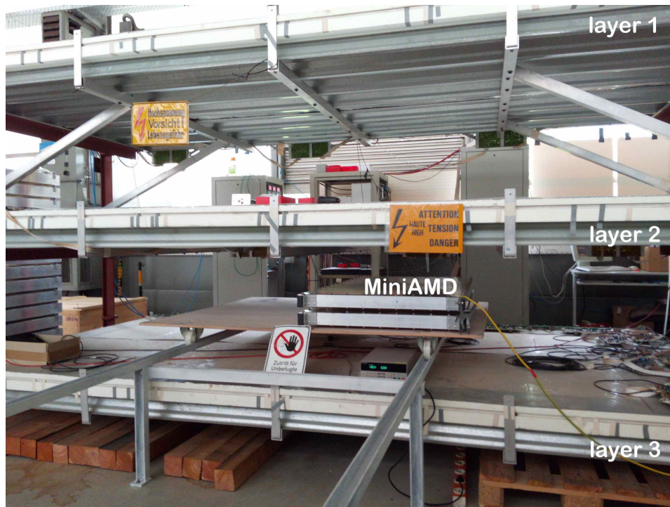
Figure 8.17.: Photo of the setup at the muon tomograph at KIT, Karlsruhe. Shown are the three layers of the tomograph. Between the two lower layers, two MiniAMD modules are located. They comprise in total 16 units of layout 2. Here, both modules are stacked. For the measurements presented, both modules are placed next to each other at the same level.
