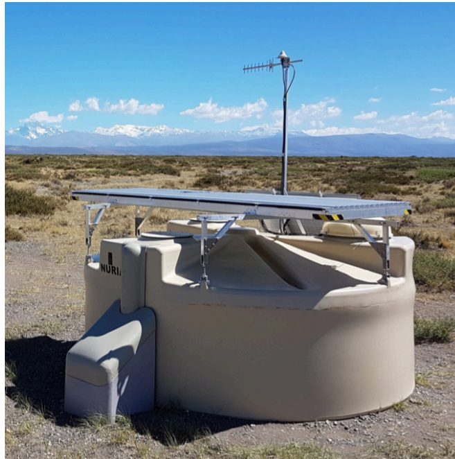
Figure 3.11.: Photo of a SSD compartment mounted on top of the water Cherenkov detector station at the Pierre Auger Observatory.
