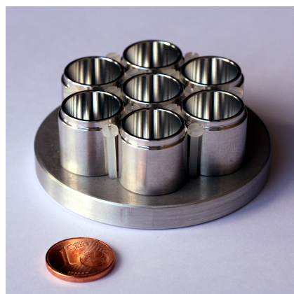
Figure 4.19: Focal plane union of FAMOUS consisting of seven hexagonally arranged Winston cones [69].
