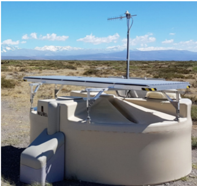
(a) One station of the AugerPrime Engineering Array with a SSD on top of the WCD.
