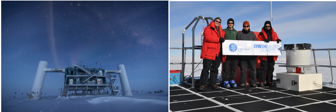
Figure 6.31: Left: photograph of the IceCube laboratory near the Scott-Amundsen South Pole station. Here, all data cables of the IceCube detector converge to the central data acquisition. The IceAct Cherenkov telescope prototype has been installed on the roof of this station in November 2015. Data taking is scheduled for the polar night beginning in May 2016. The trigger of the telescope is fed to IceCube to seek for coincidences with cosmic rays measured by the observatory [187] (image by Felipe Pedreros, IceCube/NSF). Right: photograph taken after the successful commissioning of the IceAct prototype telescope. By detecting the Cherenkov light of extensive air showers, it could provide a veto for the IceCube detector to select events from astrophysical neutrinos (image courtesy of J. Auffenberg, RWTH Aachen University).
