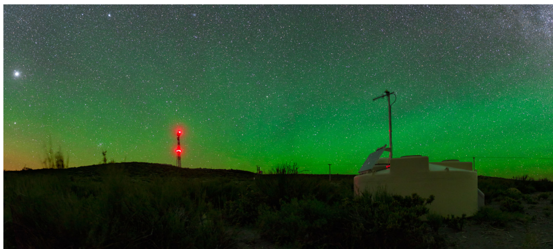
Figure 3.5: Areal photo including a water Cherenkov station of the surface detector of the Pierre Auger Observatory. Photo courtesy of S.Šaffi.
