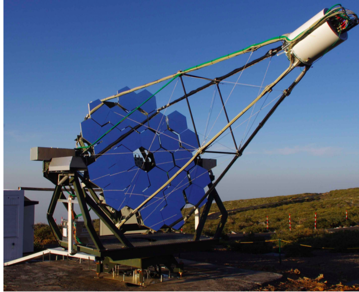
Figure 3.1 The First G-APD Cherenkov Telescope FACT is located at the Observatorio del Roque de los Muchachos on the Canary Island of La Palma. The mirror dish has a diameter of 3.8 meters. The camera made of silicon photomultipliers is located in the white cylinder in the top right corner and has a field-of-view of 4.5^\circ . Photo credit: Anderhub et al. (2013)
