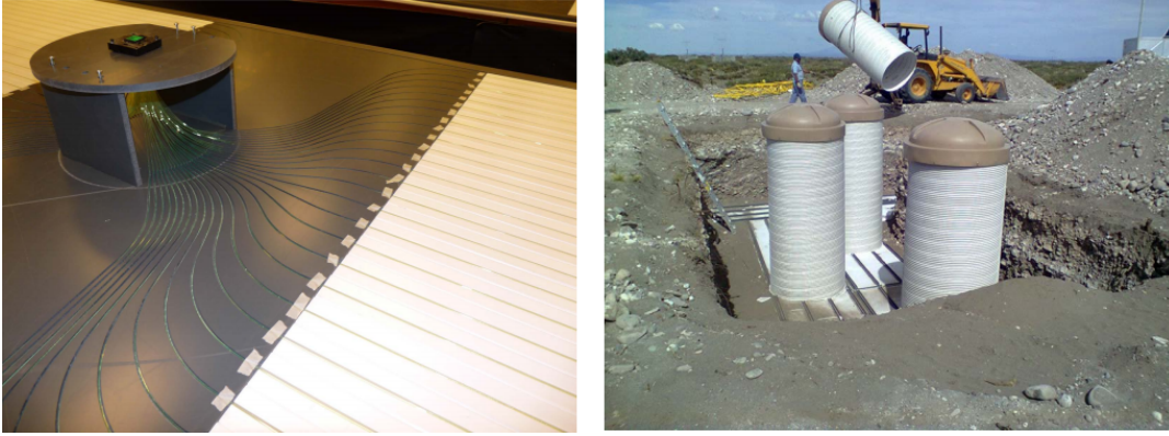
Figure 3.8.: Left: Illustration of a 10 \text{ m}^2 UMD scintillator module. The module consists of 32 scintillator bars read out with 64 optical fibres coming from each side of the module. As shown in the upper left corner the 64 fibres are concentrated to be read out in common [55]. Right: Illustration of one UMD station. The scintillator bars are placed underground. The housings contain the electronics and allow access to them. This image contains two 10 \text{ m}^2 and two 5 \text{ m}^2 modules, resulting in a total instrumented area of 30 \text{ m}^2 [55].
