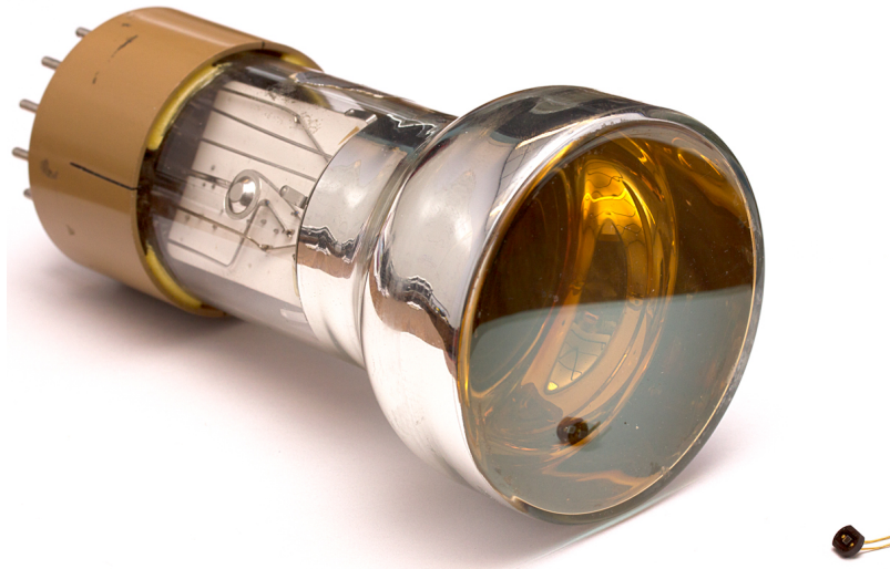
Figure 1.1: Image for comparison of the different sizes of a PMT (left) next to an SiPM (right). Taken from [1].
