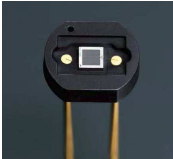
Figure 3.4: Photograph of an 1 \times 1 \text{ mm}^2 SiPM with a cell size of 100 \mu\text{m} .
