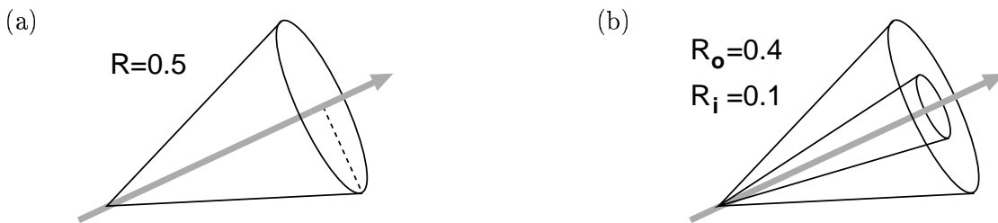
Figure 4.4: Schematic illustration of the muon isolation (a) in tracks and (b) within the calorimeter.
