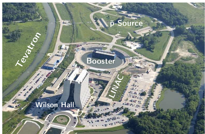
Figure 2.8: Aerial overview of the smaller accelerators at Fermilab, which are at the beginning of the chain. The LINAC, just right of the main office building (Wilson Hall), the Booster synchrotron (middle) and in the background the Antiproton Source, with its characteristic triangular shape.
