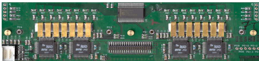
Figure 4.7: Front End Board. In the bottom part of the board the four MAD chips can be seen. [17]
