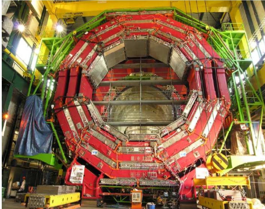
Figure 4.9: Picture of one CMS wheel equipped with drift tubes chambers and resistive plate chambers fixed on top of them (silver metallic rectangular solids) [51].
