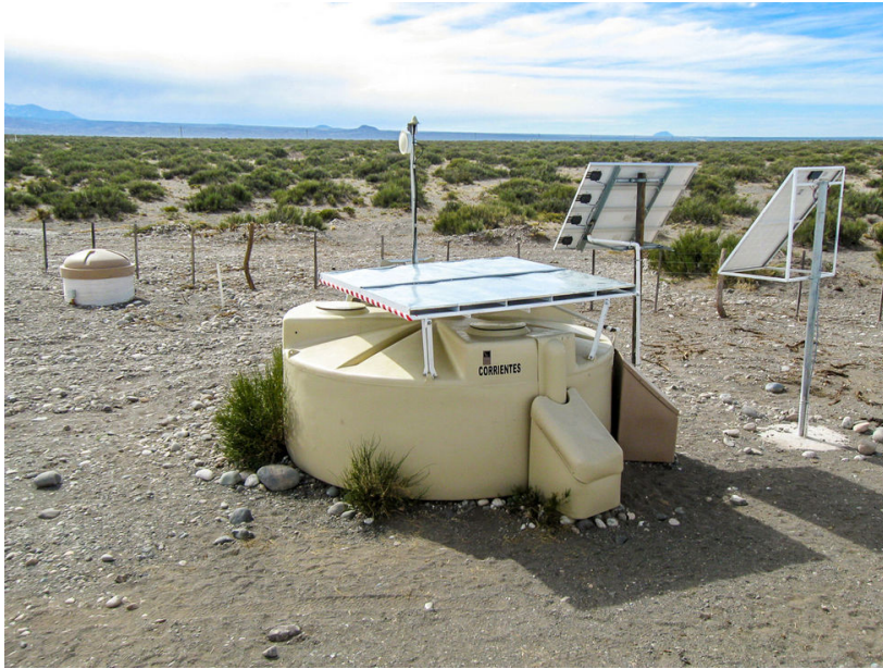
Figure 1.2: Picture of the extension of the SD station with a scintillating detector on top. Taken from [2]
