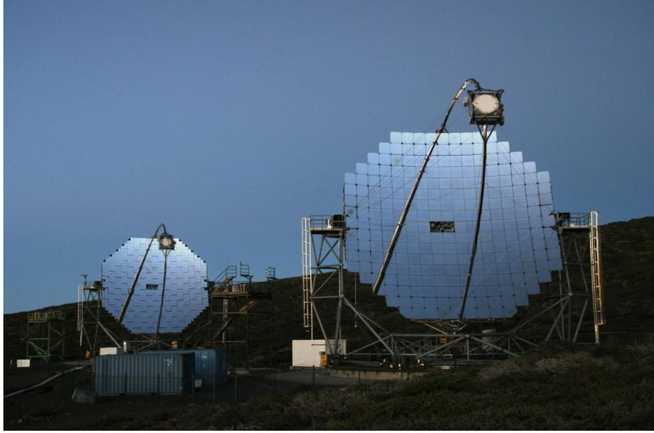
**Figure 5.1:** The two 17 m diameter MAGIC telescopes. The one in front is MAGIC-II. Taken from [77].
