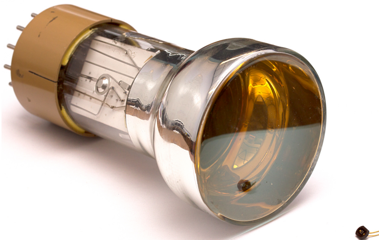
Figure 1.4.: Size comparison between a Photomultiplier Tube on the left and the SiPM as in Fig. 1.1 (Photo: Benjamin Glauß, 2012).
