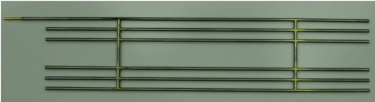
Figure 5.5.: One grid of field shaping tubes. On the upper left one can see the connector for the high voltage.
