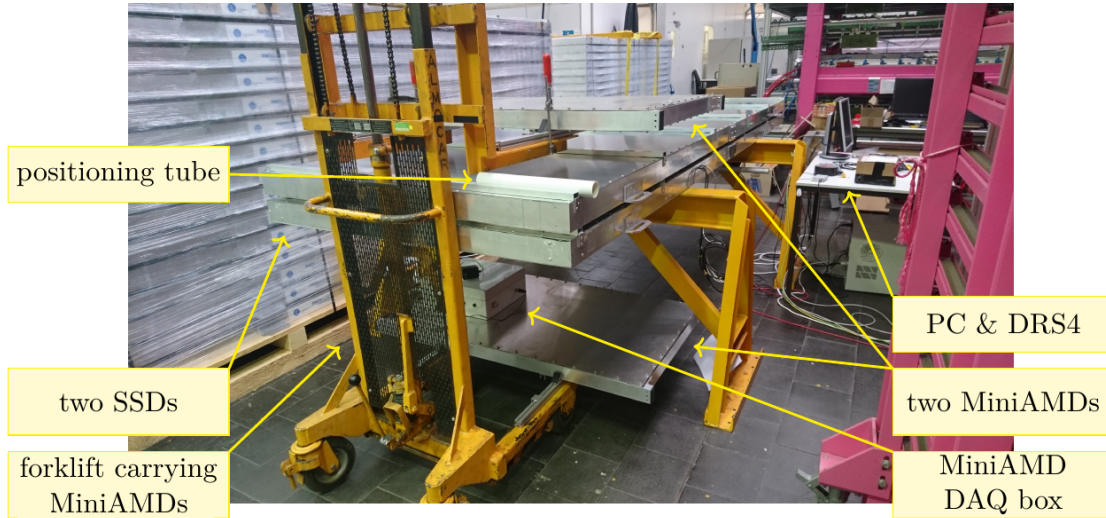
Figure 3.12. Photo of the test setup for the SSDs validations. The two MINI-AMDs are hold by a forklift. Two SSDs can be seen in the photo, but only the top one was being tested. Taken from [163].
