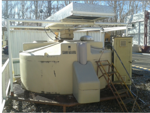
FIGURE 4.1: Picture of the experimental setup of Gianni Navarra in Malargue, Argentina. The large cylinder is the water Cherenkov station and the box on the top is one of the RPCs (the other one is not visible in this picture, since is located under the tank).
