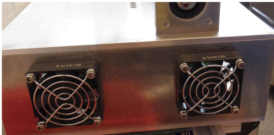
Figure 4.7: Back of the multipurpose light source with the two fans.
