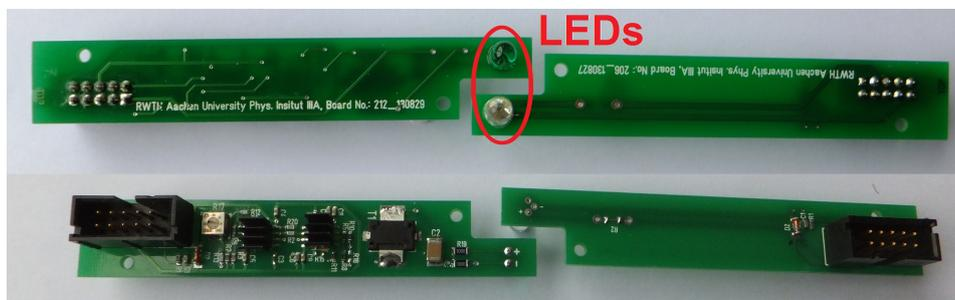
Figure 4.1: Modules as used in the multipurpose light source: Top and bottom side of the pulser module on the left and DC module on the right.
