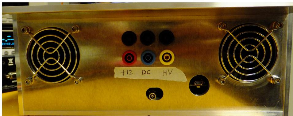
Figure 4.6: Front of the multipurpose light source. At the top there are 3 connectors for the external voltages. At the bottom there are a USB-connector and a lemo-connector for the trigger signal.
