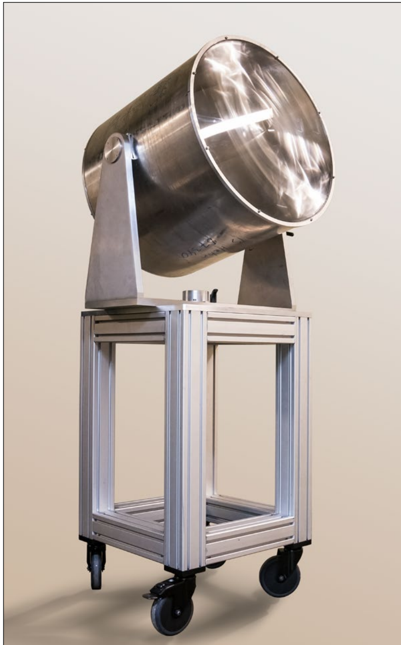
Figure 3.5: Picture of the seven pixel prototype of FAMOUS, built at the III. Physikalisches Institute A of the RWTH Aachen, which is called FAMOUS SEVEN. A Fresnel lens is mounted at the front of the telescope tubus which is attached rotatably in all directions. Photo by Tim Niggemann.
