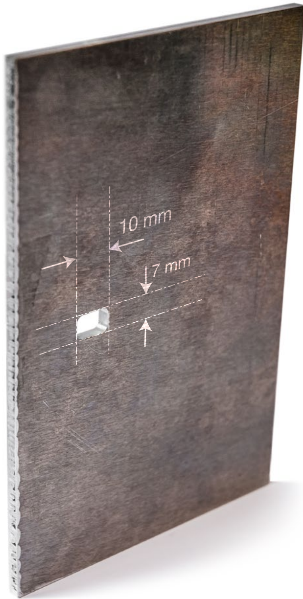
Figure 9.1: Aluminium plate with a milled window of 10 mm width and 7 mm height. The edges are rounded.
