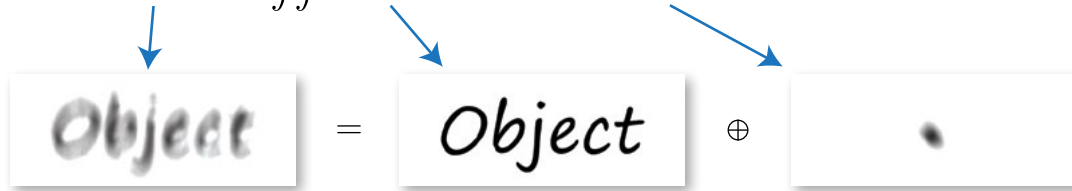
Figure 4.5: Graphical representation of equation 19: The image is formed by convolution of the original picture of the object and the PSF of the optical system. The PSF is the image of a point light source.
