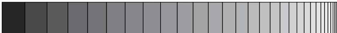
Figure 7.1: Comparison of a linear encoded brightness gradient to a gamma encoded brightness gradient. The brightness steps of the linear coding do not seem to be homogeneously distributed. Both gradients are encoded using 32 brightness levels (5 bit).
