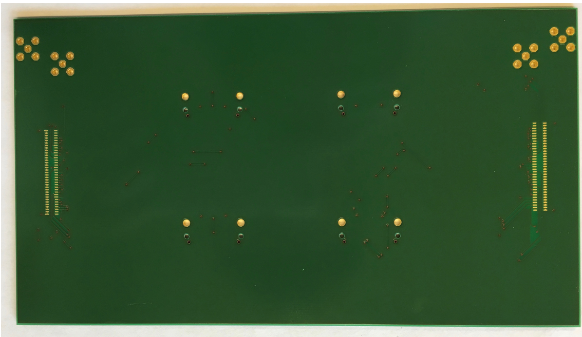
Figure 6.3: Back of the finished PCB.
