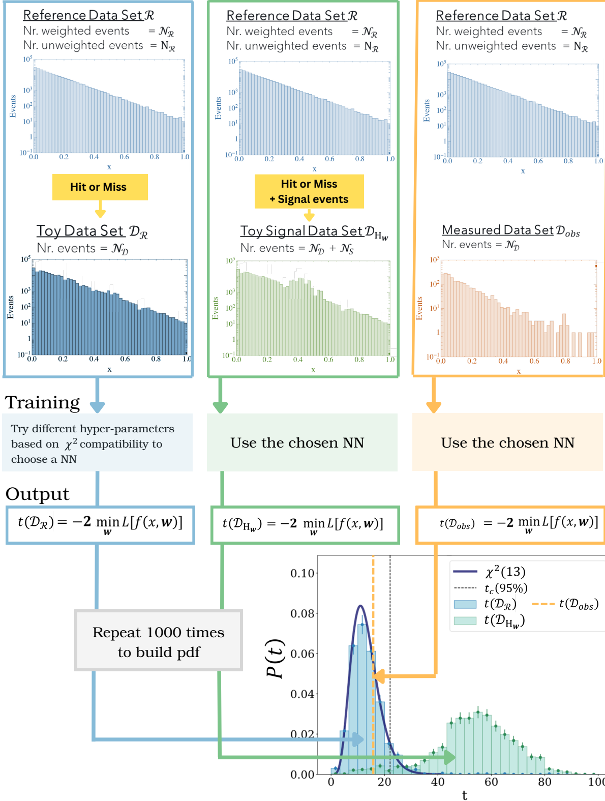
Figure 4.6: Schematic of the NPLM workflow. The blue workflow regards the comparison between the reference data set \mathcal{R} and a toy data set \mathcal{D}_{\mathcal{R}} , thrown from the reference hypothesis R using the Hit or Miss procedure. Similarly, the green workflow compares \mathcal{R} to a toy data set with added signal events \mathcal{D}_{\mathcal{S}} . Both these workflows are repeated 1000 times to build the probability distribution functions of the test statistic. Lastly, the orange workflow compares \mathcal{R} with the observed data set \mathcal{D}_{obs} . The outputted test statistic t(\mathcal{D}_{obs}) can then be used for the p -value calculation.
