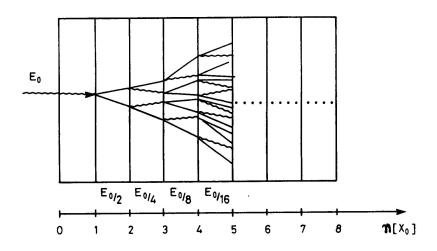
After exactly one radiation length an electron radiates and a photon splits into an electron positron pair; the energy of the primary particle is distributed equally to the two final state particles. The shower 'stops' when  $E_{\gamma} < 2m_e$  or  $E_e < E_c$  ('critical energy').
